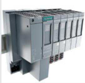
In the near future, Siemens will also offer its new EIP200S remote I/O with EtherNet/IP capability.
